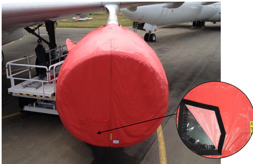
Image Above: Cambrai MVP Cover fitted to an Airbus A340 RR Trent 600 Engine
